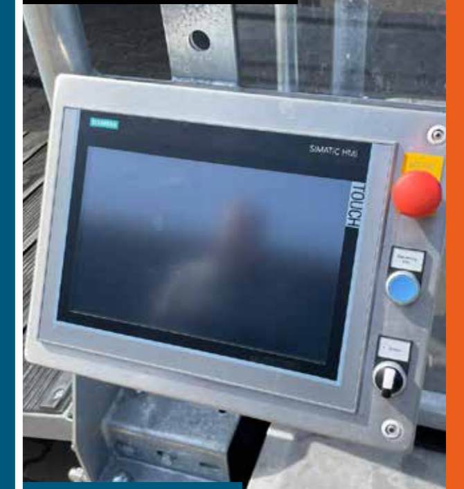
Control Panel 12" Display
